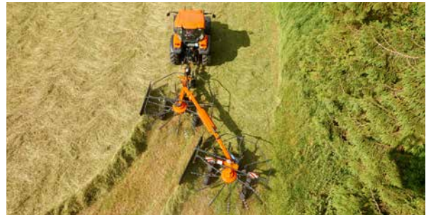
The Kubota RA2071T Vario with 7.10m working width in double swath position.
