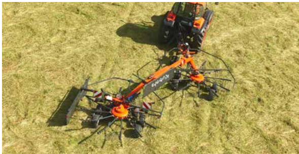
SideShift to the right - easy cleaning of borders with perfect view on the rotor.
