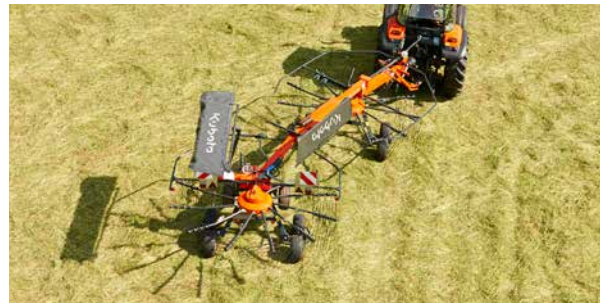
SideShift to the left - raking without driving on the crop.
