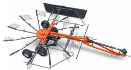
RA1047T – 4.70m working width and a weight of only 665kg.
