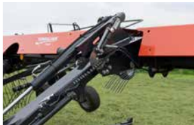
Hydraulic transport locking (optional).
