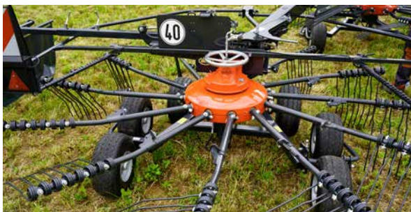
Easy adjustment of rotor height in the back.
