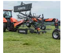
Automatic foldable swath board with parking stand.
