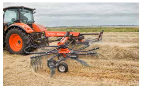
High flexibility on the road, and in the field, as no carrier frame is running on the crop.
